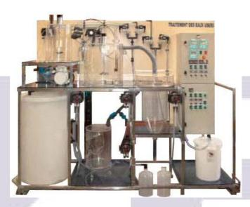
Automated Sludge Sewage Treatment Plant Model KET-102 activated sludge sewage treatment pilot plant is a small scale industrial sewage plant. It consist of all the comprehensive components and advance process control instrument to make the trainer more interesting on study.
